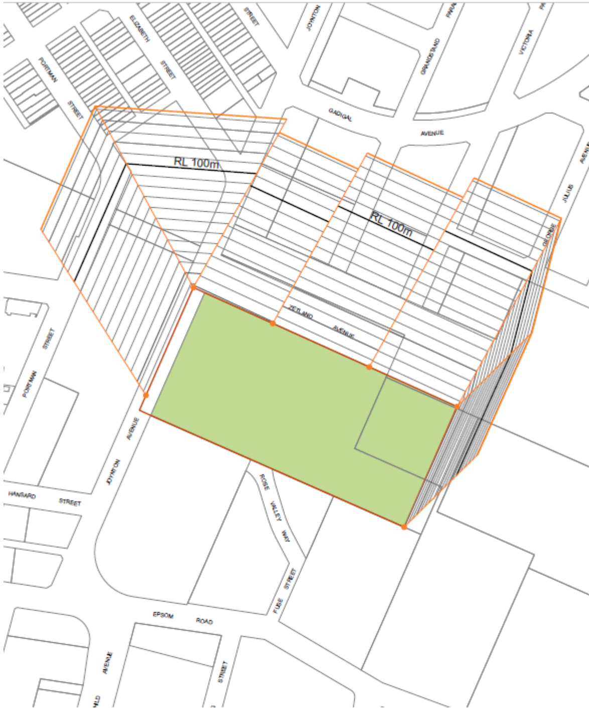
Figure 5.XXX Gunyama Park Sun Access Plane ● Node of SAP — Ray ascending edge — RL 100m Contour — RL 50m Contour — RL 5m Contours
